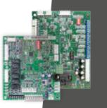
full two way communication between components, advanced operating logic and robust troubleshooting capabilities. It carries support for true energy monitoring, extended hot water generation control and integration with our IntelliZone2 zoning system. Incorporating the upcoming Aurora Web Link (AWL) module also extends communication protocols to include the internet, smart grids, home automation networks and more.
